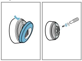
Open the cooking sensor lid and remove the battery from the base.
