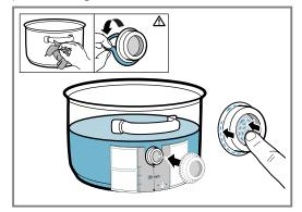
3. Press down all over the surface of the silicone patch, including in the centre.
